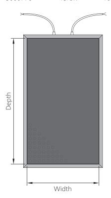
According to ISO 13855, the minimum depth to the danger zone must be taken into account (see Chapter Calculation of the necessary actuation area). The non-sensitive edges must be taken into account (see Chapter Non-sensitive edges).
